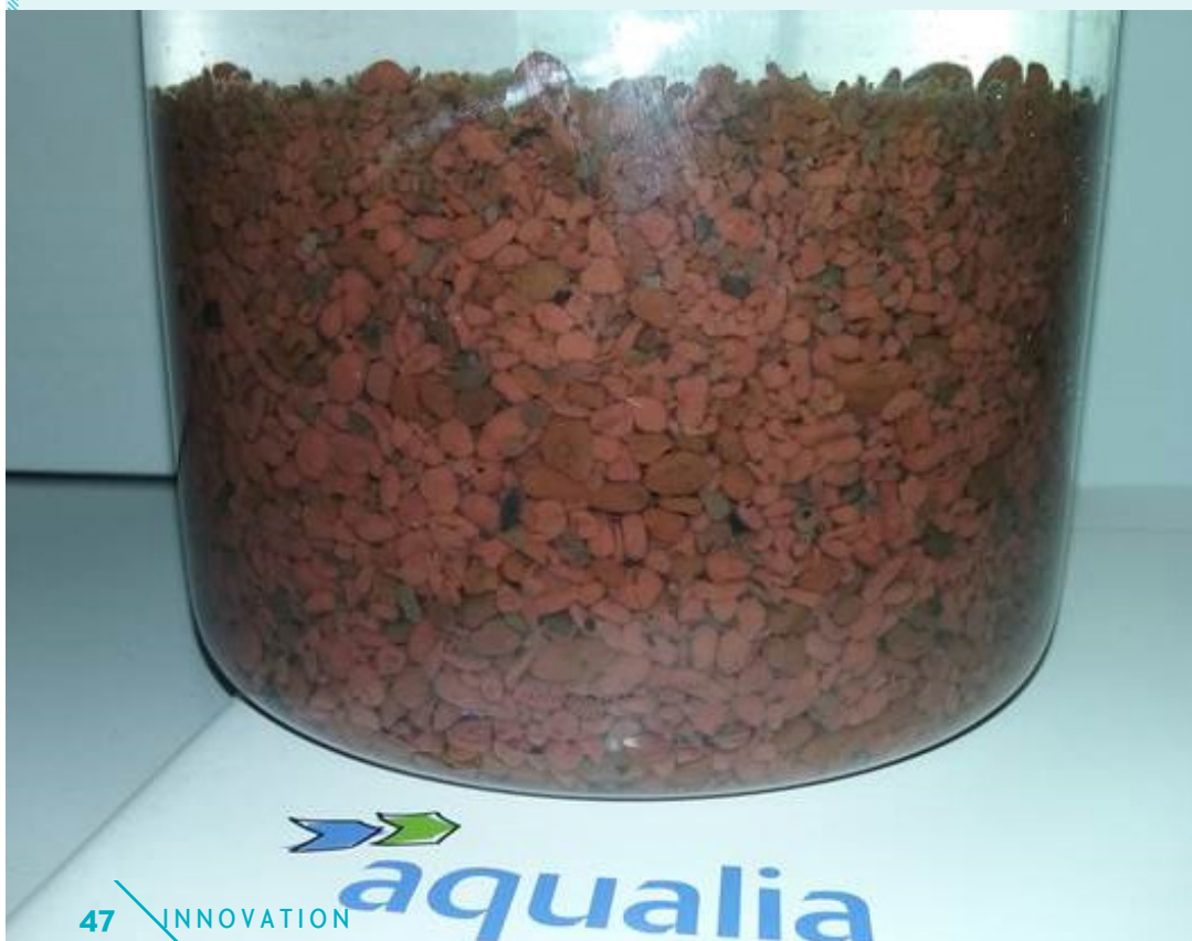
The granular ELAN®-ANAMMOX biomass at the pilot facility
