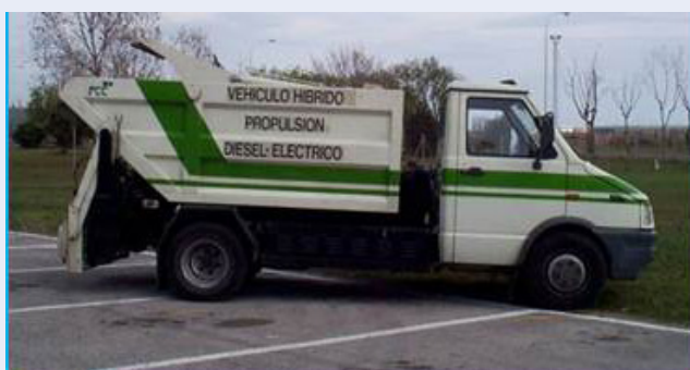
Compacar 3500, electricity-driven and self-charging battery
